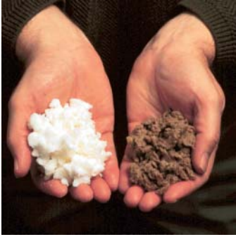
Naturally dark brown wood pulp (right) is useful for making paper bags and boxes. After bleaching and softening (left) pulp produces higher grades of paper and other products.
