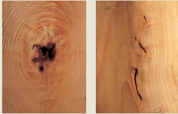
Veneer is usually made from the "highest quality" logs. Defects and imperfections such as knots and decay (above) make veneer unusable.
