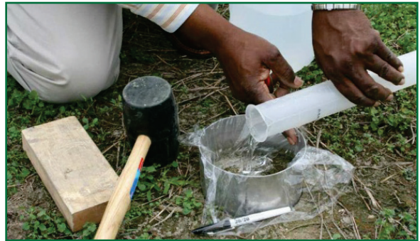
Figure 1. Water is poured into plastic-lined ring.
